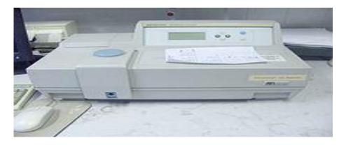
A spectrophotometer is an apparatus used to measure the amount of photons converted into electric current that can measure intensity as a function of the light source wavelength.
